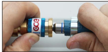
1. Pull the "blue" sleeve of the Quick connector and insert the coupling pin into the Quick connector.
