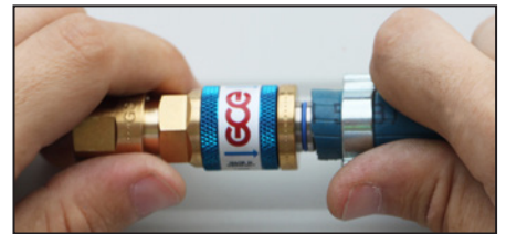
1. Mounting is finished. O-ring is visible.
